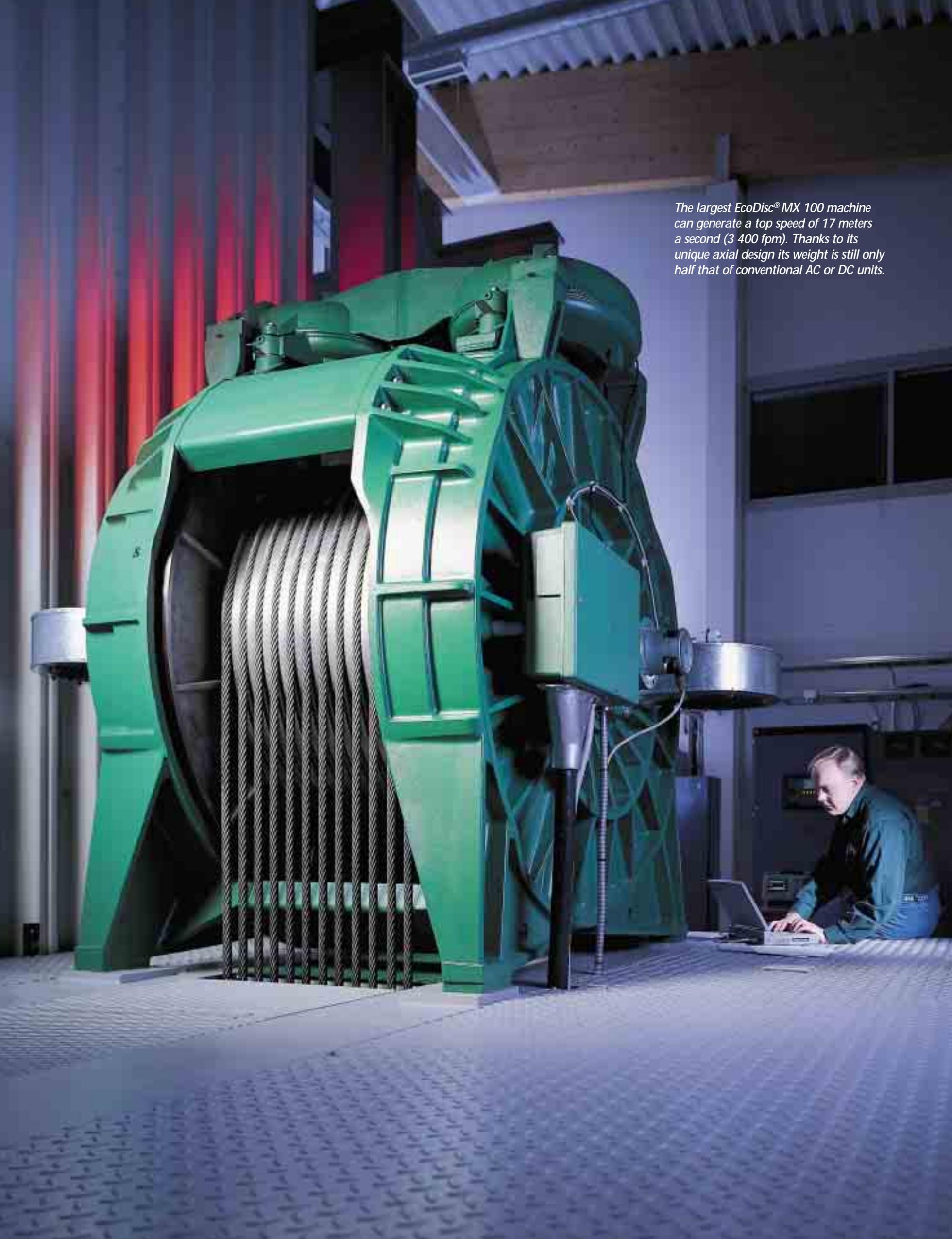
*The largest EcoDisc® MX 100 machine can generate a top speed of 17 meters a second (3 400 fpm). Thanks to its unique axial design its weight is still only half that of conventional AC or DC units.*
