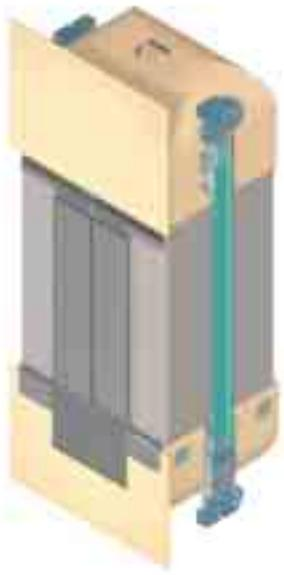
*The insulated, double-wall Alta™ car enclosure eliminates up to 25dB(A) of hoistway noise and features 'tuned' ventilation. The door panels are fully insulated. Sealed door panel edges prevent air leaks and noise. The heavy-duty door operator uses the same PMSM technology as the hoisting units.*
