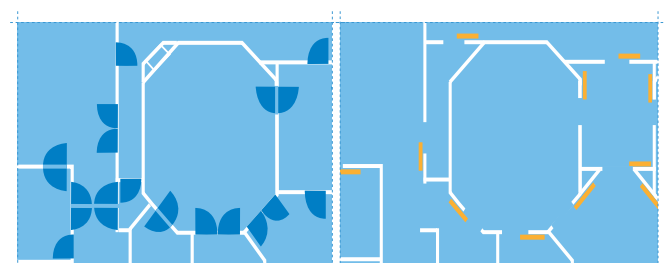
Gliding vs swing doors can save up to 15% of space based on opening area that swing doors require
