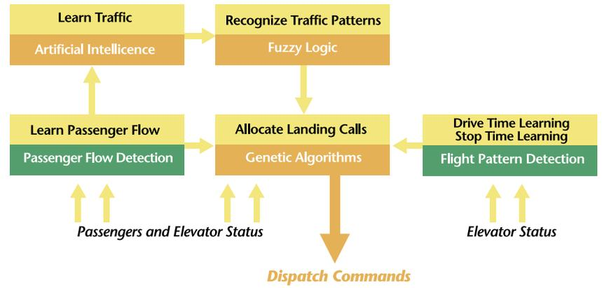
The group controller uses the fast Genetic Algorithm protocol that generates best dispatching solutions in all traffic situations.
